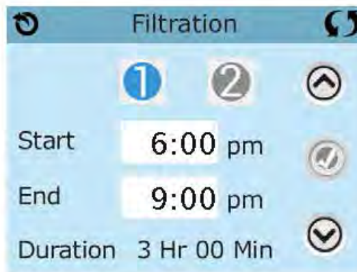
Viewing Filter 1 while Filter 2 is ON:
